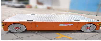
Figure 3: Omnidirectional mobile platform with Mecanum wheel.
